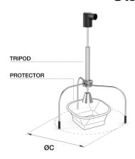
The JBC Hot Air stations use jointly protectors and tripods for a faster and more comfortable desoldering job.
