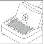
The softest cleaning method. Keep the sponge damp with distilled water when working to avoid tip wear.
