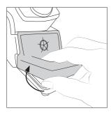
Lift the wiper at its front edge.
