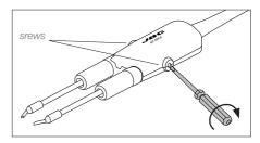
Lock the fixing screws.
