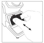
Replace the brass wool with a new one when it is worn out. Place the wiper back o replace them if desired.
