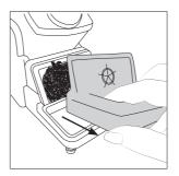
Remove the wiper by pulling it out.
