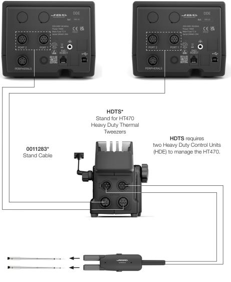
C470\* Cartridges HT470 Heavy Duty Thermal Tweezers
