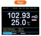
GOM-804/805 has two measurement speed selections, which are Fast reaching 60 readings per second, and Slow 10 readings per second. A major departure from the past, users, in the past, had to juggle between speed and display resolution. GOM-804/805 will not affect resolution despite of any speed selections and will maintain the highest display digits. In other words, reading resolution will not be changed by changing speed and the display digits remain the same.
