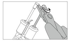
Align cartridges with JBC pliers.
